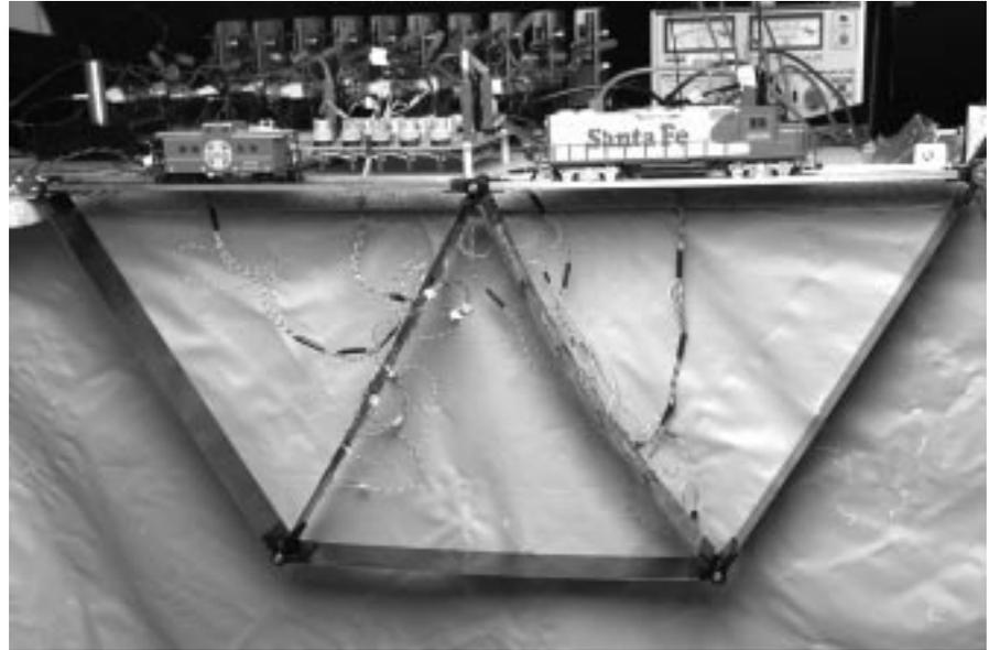
**Figure 7: Actively stabilized truss bridge.** This bridge incorporates two compressive members that actively resist buckling.
