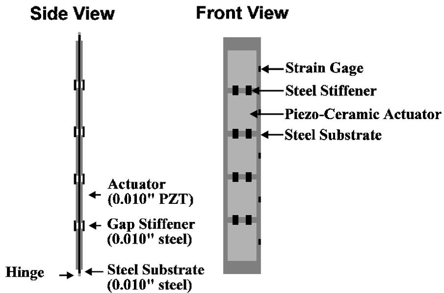
**Figure 3: Front and side views of the composite steel/piezo-ceramic column.** The column is 12.6 inches in length. Steel stiffeners are used to increase the stiffness of the area between adjacent actuators that is not covered by piezo-ceramic material.
