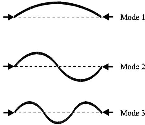
**Figure 1:** The first three mode shapes of a beam with pinned ends, as determined by Equation 1. The shape of the beam at any instant in time is expressed as a sum of mode shapes. The amplitude of each mode shape varies with time as determined by Equation 2.
